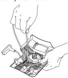
Remove any remnants of the old starter cord and check that the return spring works. Insert the new starter cord through the hole in the starter housing and in the cord pulley.
